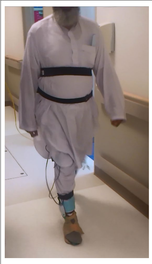
Figure 3. To access the accuracy of SmartSox in measuring parameters of interest, participants were asked to walk a distance of 30 m as comfortable speed while wearing SmartSox. Computerized plantar pressure insoles (F-Scan®, Tekscan, Inc, Boston, MA, USA) were used as a reference to validate the accuracy of SmartSox to measure plantar pressure. Thermal stress response was measured using a thermography. To control number of taken steps, a validated gait analyzer based on wearable sensors (LEGSys™, Biosensics LLC, Boston, MA, USA) was used.
