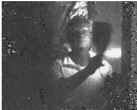
Fig. 6. Short-wave infrared image taken using the nano-injection imager. The nano-injection imager is cooled to 200 K. The subject was standing in a completely dark room, holding a soldering iron at around 350 °C.
