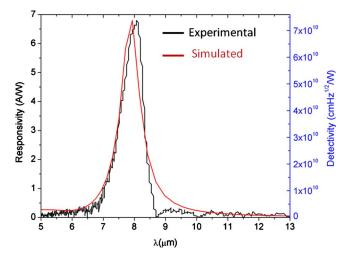
FIG. 5. (Color online) The measured responsivity (left) and detectivity (right) spectrum of the device at a normal-incident infrared radiation at the bias of 0.7 V at 78 K (the black curve) and the simulated averaged  $E_z$  intensity spectrum (the red curve) in the quantum well active region.
