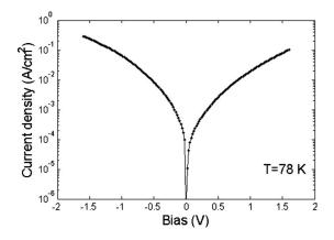
FIG. 4. The measured dark current density-voltage curve of the device at 78 K.
