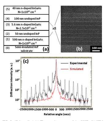
FIG. 2. (Color online) (a) The growth structure of the QWIP; (b) SEM image of eight periods of quantum well active regions (the brighter region is the doped InGaAs layers); (c) simulated and experimental XRD curves of eight periods of quantum wells.
